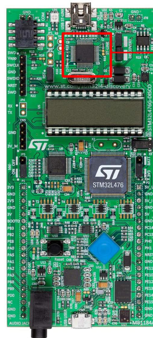
Integrated ST-Link/V2 programming and debugging tool
