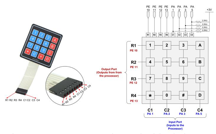
The maximum current a GPIO pin can source or sink is 20 mA. When calculating the value of external pull-up resisters, make sure that the current should not exceed 20 mA.
